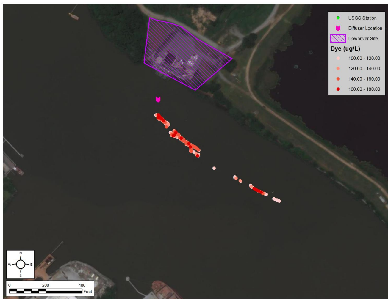
Figure 10-12 Front River Dye Sampling – August 25, 2020 (mid-depth) (100 to 180 \mu\text{g/L} )
