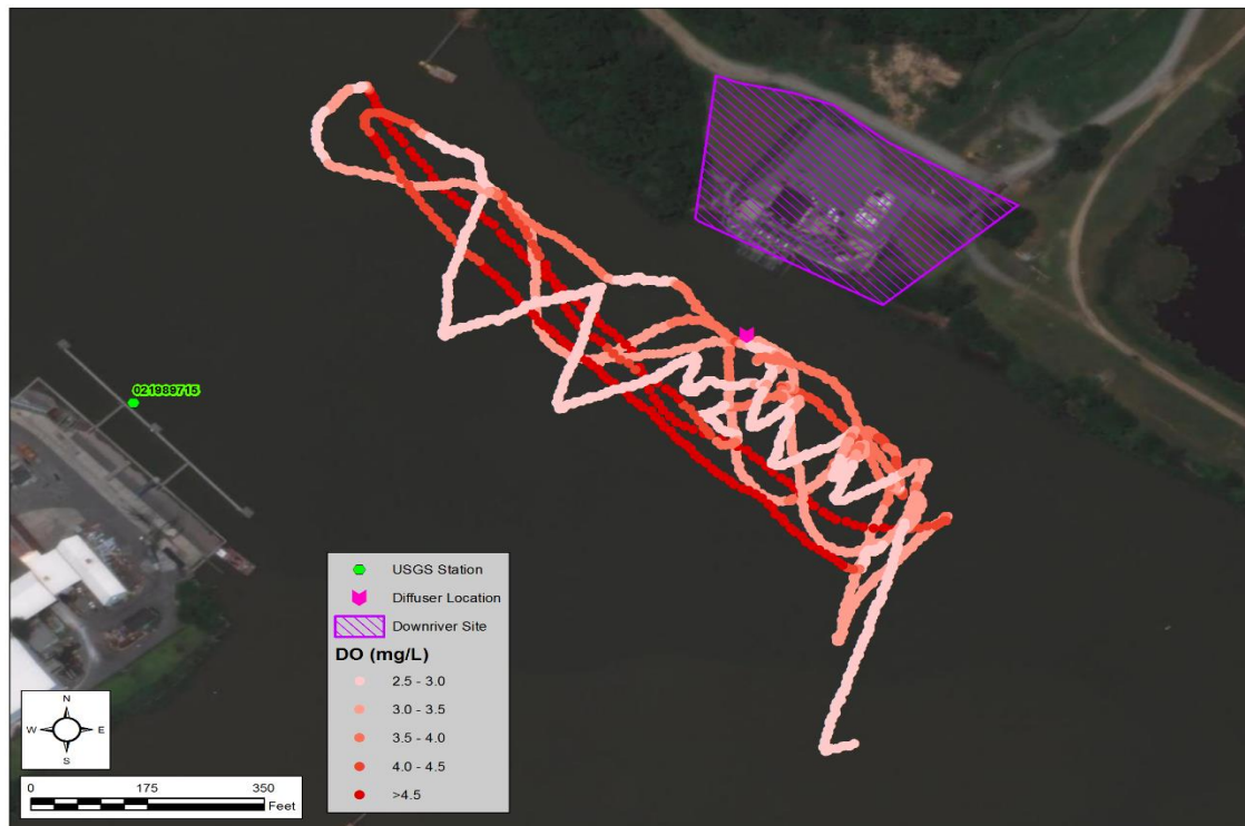
Figure 9-2 Front River Drift Sampling – August 17, 2020 (mid-depth)
